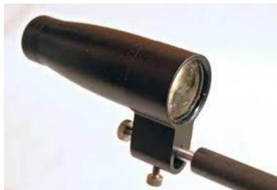
or simply using the old eyeball bore-sighting method, it is almost invariably possible to get the windage correct without using the windage adjustment in the scope at all. By slackening one side and tightening the other, you will be able to get the windage just where you want it with the internal adjustment still in the ideal central position. Once you have completed this
